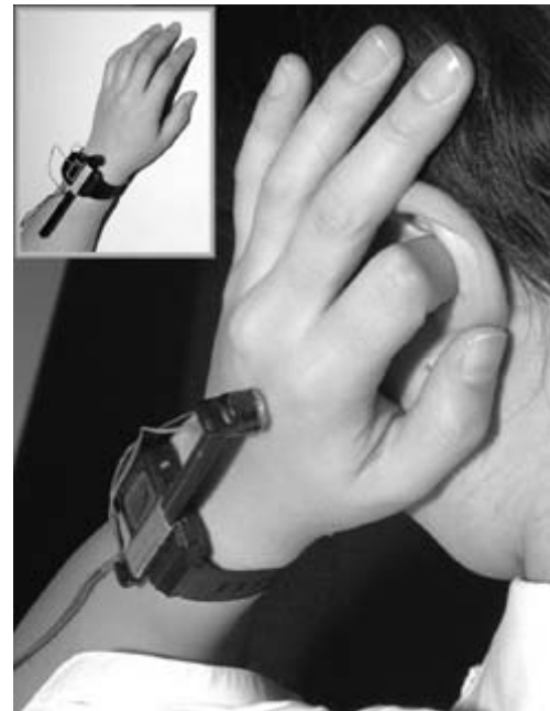
Figure 3: Whisper (boom actuator) When operating, the boom is pulled out, and the user's hand is bent backwards.
