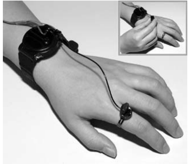
Figure 2: Whisper (ring actuator) Hook switch is built into the cord-reel, and it turns on when the electrical wire is pulled.
