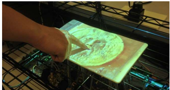
Figure 1. VacuumTouch: user can feel the attractive force to the surface without requiring holding or attaching an additional device. Here, user is feeling the attractive force from La Bocca della Verità.
