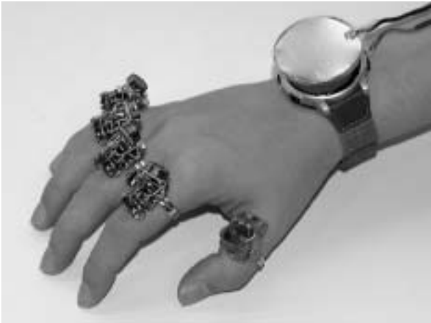
Figure 5: Wireless FingerRing (prototype). Size of TX will be reduced by the use of specially manufactured IC chip.
