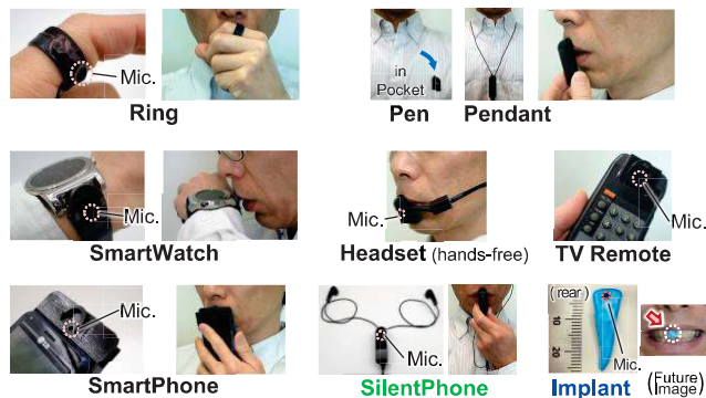
Figure 7: Variations of SilentVoice devices
