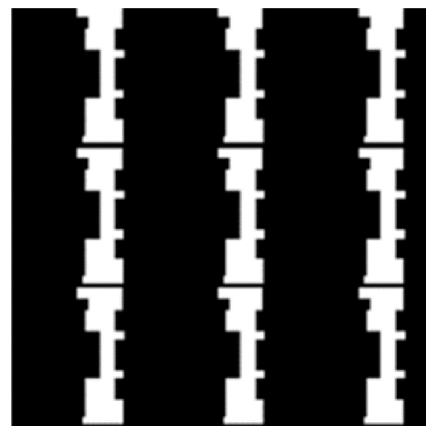
Figure 1. Image of 3x3 pixels of proposed 4K tOLED structure. White regions are clear on the design. Pixel pitch is 315 \mu\text{m} .
